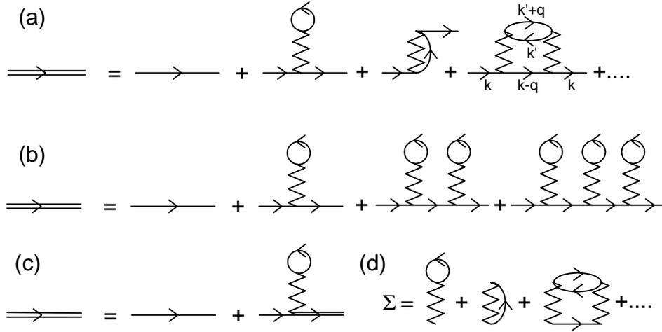
Figure 2: (a) The first few diagrams in the Fermion perturbation expansion. (b) A selected set of diagrams to infinite order. (c) The sum of (b) can be done diagrammatically:  $G = G^0 + G^0 \Sigma_H G$  with  $\Sigma_H$  the “potential + closed fermion loop” diagram. (d) Expansion for the self energy  $\Sigma = \Sigma_H + \dots$ . The labels are to be read as “4-vectors”, i.e.  $k \equiv \vec{k}, \omega$ .
