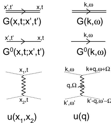
Figure 1: Dictionary for Feynman diagrams.  $G$  is the propagator of the interacting system;  $G^0$  that of the noninteracting system; and  $u$  is the pairwise interaction (the dotted lines show where the propagators are to be attached).
