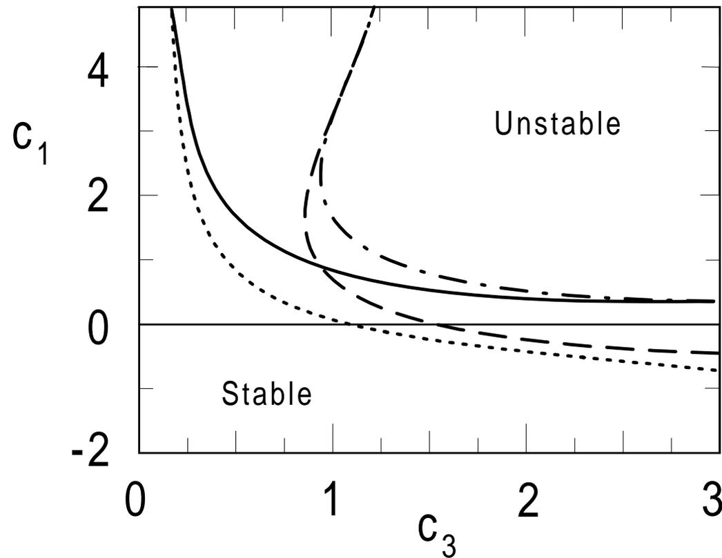
Stability lines of the CGLE. Solid line: Newell criterion  $c_1 c_3 = 1$ ; dotted line: (convective) Benjamin-Feir instability of spiral-selected wavenumber; dashed: absolute instability of spiral selected wavenumber; dashed-dotted: absolute instability of whole wavenumber band. Unstable states are towards larger positive  $c_1 c_3$ .
