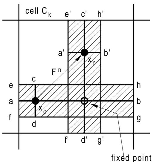
Figure 22.2: Point  $x_0$  is mapped into  $x_n$  under  $F^n$ . Then if  $ab \rightarrow a'b'$  and  $cd \rightarrow c'd'$  the parallelogram  $efgh \rightarrow e'f'g'h'$ , and by continuity there must be a single saddle fixed point of  $F^n$  in the intersection region. In all cases the horizontal (vertical) lines in the figure are segments of the stable (unstable) manifolds. The figure is drawn with orthogonal lines for simplicity, but this is not essential to the argument.
