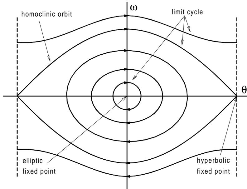
Figure 2.1: Phase space of the ideal pendulum
