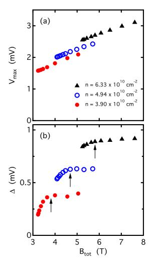
FIG. 3. Effect of in-plane magnetic field on  $\nu=1/2$  tunneling critical points,  $V_{\rm max}$  and  $\Delta$ , at three different densities, plotted versus total magnetic field  $B_{\rm tot}$ . For each density, the perpendicular field  $B_{\perp}$  is fixed while the in-plane field  $B_{||}$  is varied. The leftmost data point of each set corresponds to  $B_{||}=0$  (tilt angle  $\theta=0$ ). The arrows indicate our assignment of the "knee" in the  $\Delta$  vs  $B_{\rm tot}$  data.
