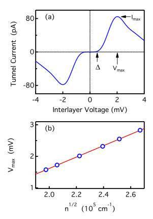
FIG. 1. (a) Typical tunneling IV characteristic at  $\nu=1/2$ . Data taken at T=50 mK with  $B_{\perp}=4.09$  T and  $B_{||}=0$ .  $I_{\rm max}$  and  $V_{\rm max}$  denote location of maximum tunneling, while  $\Delta$  is voltage where tunneling current has reached  $0.02I_{\rm max}$ . (b) Density dependence of  $V_{\rm max}$  at  $B_{||}=0$ . Solid line is an unweighted least-squares fit of  $V_{\rm max}$  versus  $n^{1/2}$ ; the fit extrapolates to  $V_{\rm ex}=-2.0$  mV at n=0.
