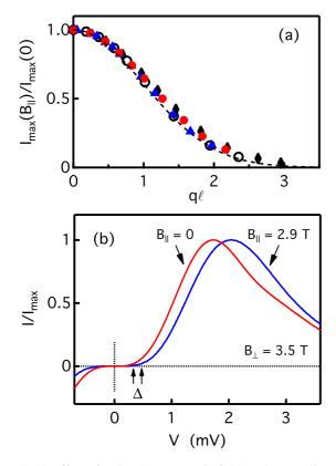
FIG. 2. Effect of an in-plane magnetic field on the tunneling IV curve at  $\nu=1/2$ . (a) Maximum tunneling current versus  $q\ell$  at various densities. Dashed line is theory prediction described in text. (b) Normalized  $\nu=1/2$  tunneling IV curves at  $n=4.24\times 10^{10}$  cm<sup>-2</sup> for  $B_{||}=0$  and  $B_{||}=2.9$  T. Upward arrows near lower left show change in  $\Delta$  induced by the in-plane field. Data taken at T=50 mK.
