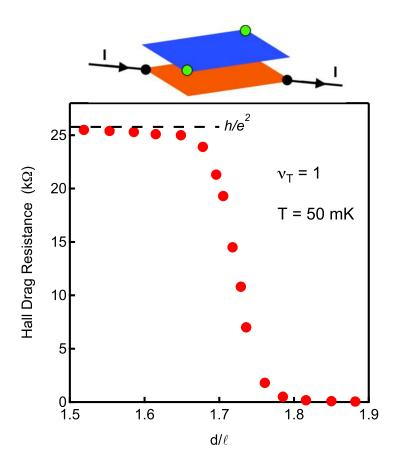
FIG. 7: Quantization of Hall drag at  $\nu_T = 1$ . Drawing depicts idealized Hall drag set-up in a simply-connected, square geometry. Current flows only through lower layer, while Hall voltage is measured across opposite layer (via the green contacts). Data shows development of Hall drag resistance quantization to  $R_{xy,D} = h/e^2$  as  $d/\ell$  is reduced. After Kellogg *et al.* [28, 90].
