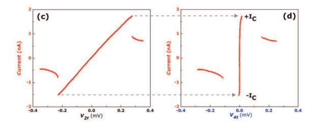
FIG. 5: Tunneling at  $\nu_T = 1$ . Left panel: Two-terminal IV characteristic. Linear segment around V = 0 implies a series resistance of roughly 150 k $\Omega$ . Instability at  $\pm 1.6$  nA is clearly evident. Right panel: Four-terminal IV reveals the Josephson-like jump in the tunneling current at  $V_{4pt} = 0$ . After Tiemann  $et\ al.\ [46]$
