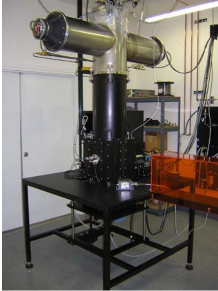
Combustion test section with acoustic forcing system.
