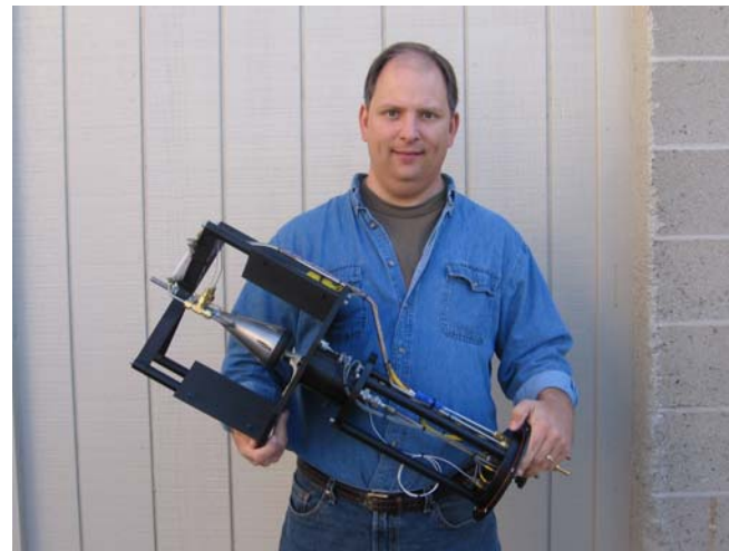
Nd:YAG pump laser and custom built optical parametric oscillator (OPO).
