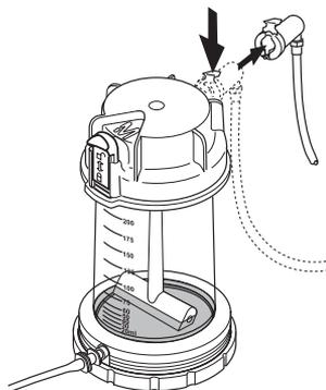
4. Unscrew cap and remove from cell body.
