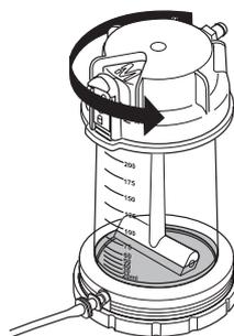
5. Remove stir bar and recover concentrated sample. Save filtrate sample if required.
