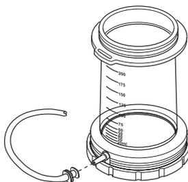
5. Insert stir bar into cell body until support ring is seated on ridge inside the top of cell body.
