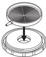
2. Place membrane into membrane holder, oriented as indicated in membrane instructions. Place O-ring on top of membrane and push down gently to seat membrane in holder.
