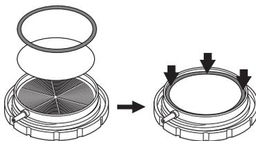
3. Align filtrate port on membrane holder with slot in bottom of cell body. Screw base into cell body.
