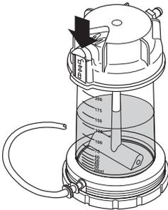
10. Attach pressure inlet tubing assembly by inserting female connector onto quick-connect fitting on cap until it clicks.
