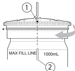
1. Tighten the cap/closure until this mark is as closely as possible aligned with the bottle vent line
