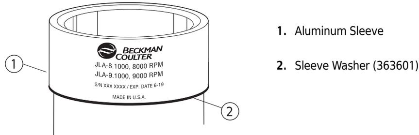
New canisters can be used with the same rotor body.
