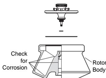
Periodically (at least monthly) inspect the rotor body for rough spots or pitting, white powder deposits—frequently aluminum oxide—or heavy discoloration. If any of these signs are evident, do not use the rotor. Contact your Beckman Coulter representative for information about the Field Rotor Inspection Program (FRIP) and the rotor repair center.
