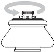
1. Place one hand on the rotor to keep it from turning. Grasp the tie-down knob with your other hand and turn it to the left (counterclockwise), while pulling up, until the stem disengages from the drive hub.
