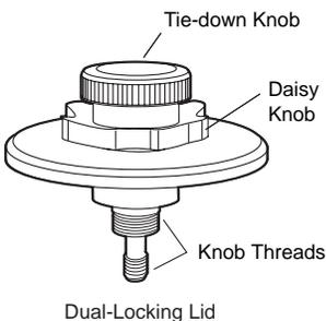
1. To prevent the rotor from sticking to the centrifuge drive hub, apply a thin coat of Spinkote lubricant to the rotor drive pins and to the lid knob threads.
