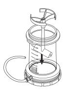
7. With cap oriented as shown, seat large diameter of gasket in gasket groove. Gently push the gasket down to seat it fully.
