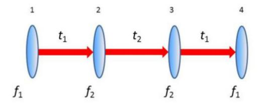
For the first and last lenses (1 and 4), we will use 200 mm focal length, 50 mm diameter achromatic doublets composed of BK7 and SF2 glasses. For the center two lenses (2 and 3), we will use 75 mm focal length, 50 mm diameter achromatic doublets composed of SF11 and BAF11 glasses. All doublets were off-the-shelf catalogue optics from Thorlabs (Table 1) and had anti-reflection coating in the visible spectrum. Total length of the system is 910 mm.
