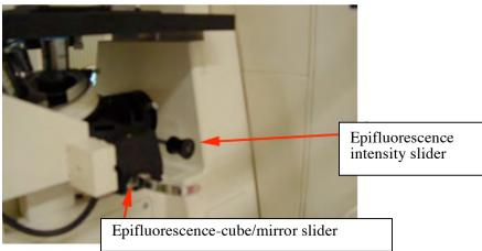
**B)** Check Epifluorescence Intensity Slider Directly behind the epifluorescence filter cube is a slider that controls if and how much light from the mercury source reaches the stage. When the slider is pulled to the far right it blocks all light, the middle and left positions are empty allowing light to pass through.
