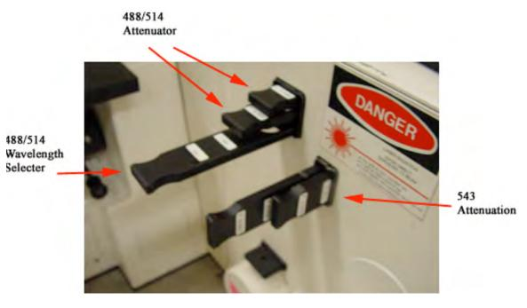
In "At" menu, set the left column to 1 and the right column to the number that matches the total laser line attenuation that results from the chosen attenuator positions (see tables below).
