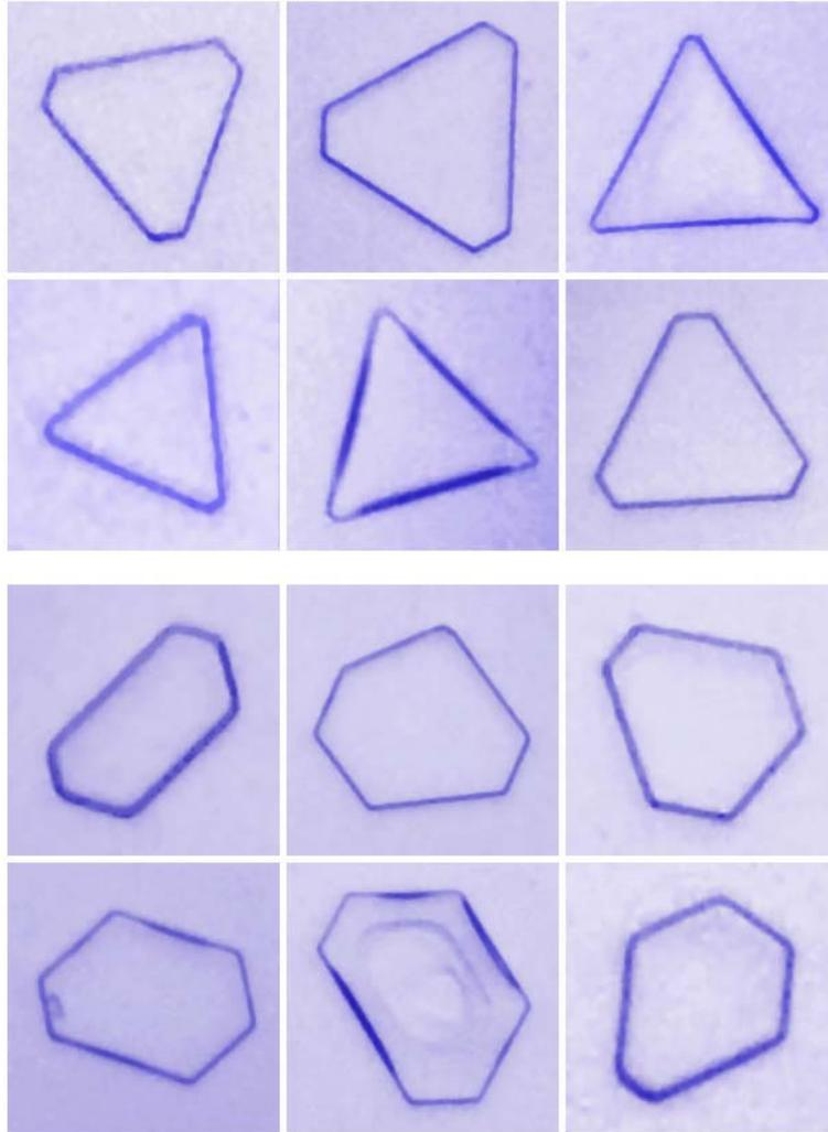
Figure 4. Examples of some extreme ( $H < 1/3$ ) crystal morphologies seen in our data. The top six images show crystals with  $T < 1/2$ , while the bottom six show crystals with  $T > 1/2$ . The former were much more common than the latter, as can be seen from Figure 3. Equivalent diameters ranged from roughly 50 to 100 microns.
