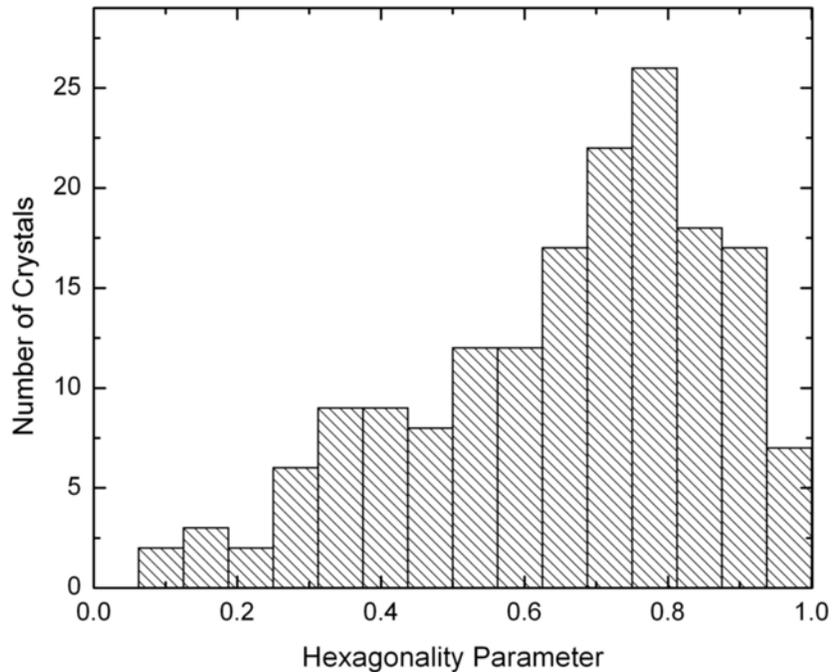
Figure 2. Distribution of laboratory-grown crystals as a function of the hexagonality parameter  $H$  defined in the text. These data are from an unbiased sample of plate-like crystals grown at  $-10$  C with a water vapor supersaturation of 1.4 percent.
