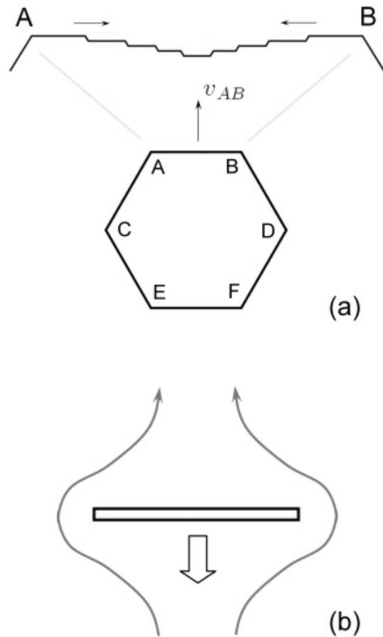
Figure 5. (a) The formation of facets in a simple hexagonal plate-like crystal, as described in the text. The top figure shows a close-up of the  $AB$  facet, exaggerated to show molecular steps on the surface. (b) A schematic depiction of airflow around a falling hexagonal plate crystal (seen from the side).
